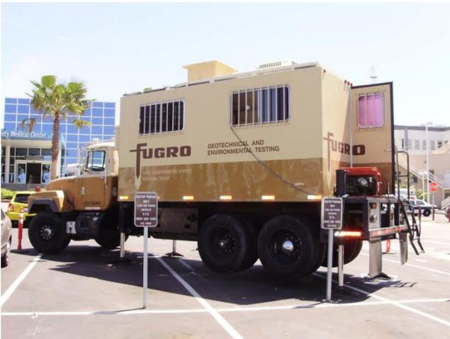
Cone Penetration Test (CPT) Truck
